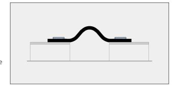
At higher pressures (1 bar) and greater diameters ( $> \varnothing 500$  mm), the fixing of a sleeve expansion joint may lead to sealing problems. There is also the risk that the expansion joint will be pulled off the pipeline. For this reason, we recommend that you attach a welding bead or a wire to the pipeline ends.
