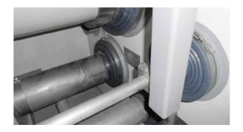
Following a dose of 200 kGy from ionised radiation the rubber elasticity remains to 200 %
