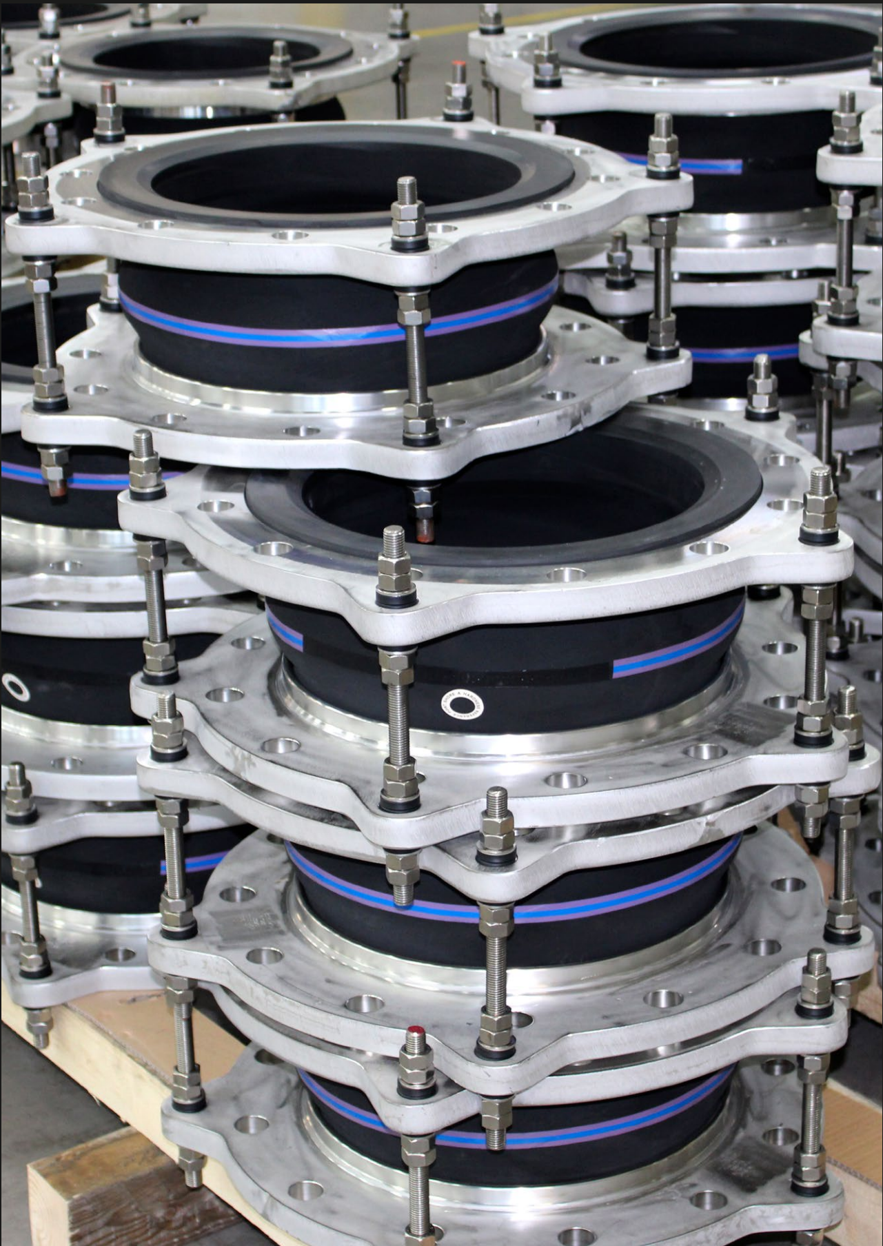
D112M lateral FPM rubber expansion joints of size Ø 400 mm with embedded vacuum ring and stainless backing flanges, tie-rods and bearings
