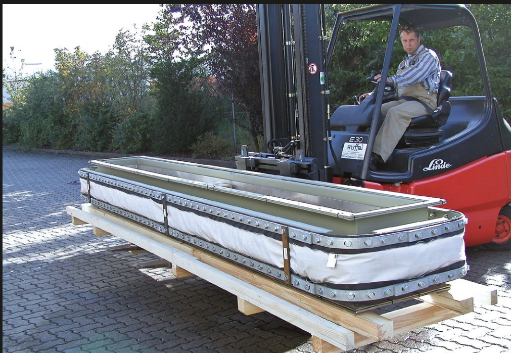
Multilayer expansion joint, type GB300 as a pre-fabricated installation unit for ash discharge in a power plant Ø 5,500 x 600 mm, 750°C
