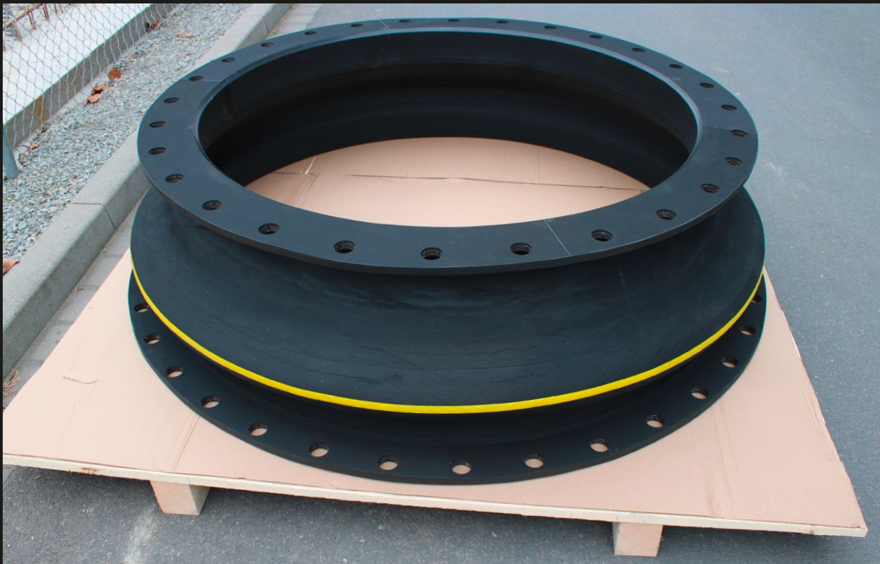
Single arch reducer made from NBR rubber with embedded vacuum ring, type U112A Ø 1,400 mm / Ø 1,200 mm, design pressure 5 bar
