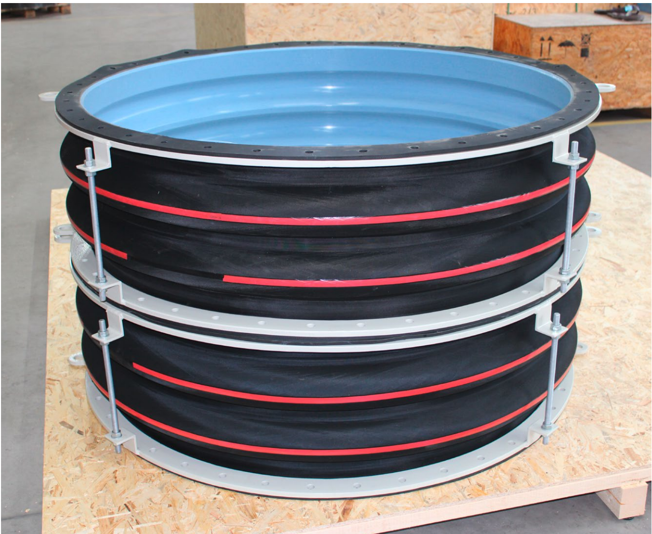
Double arch EPDM rubber expansion joints with PTFE lining for GRP gas ducts of a sulphuric acid plant as dismantling joint
