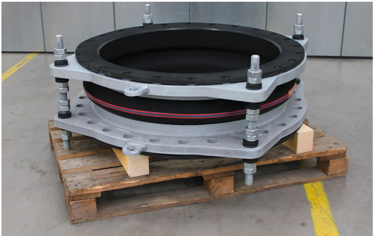
EPDM rubber expansion joint Ø 900 mm PN 16 designed according PED 2014/68/EU with aramid cord reinforcements, design temperature 120° C
