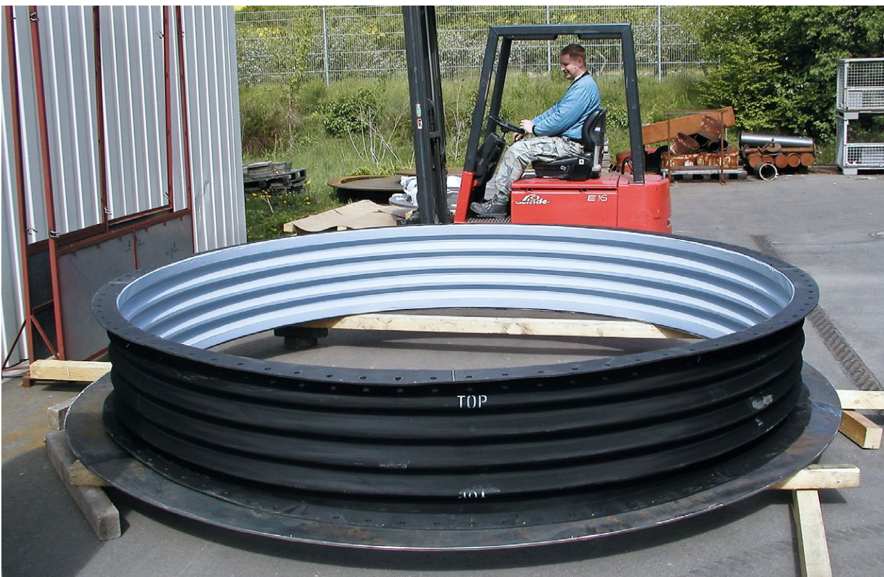
Universal expansion joint, type U142A with PTFE lining for a sulphuric acid reclamation plant Ø 2,800 mm, -0.15 bar, 80°C
