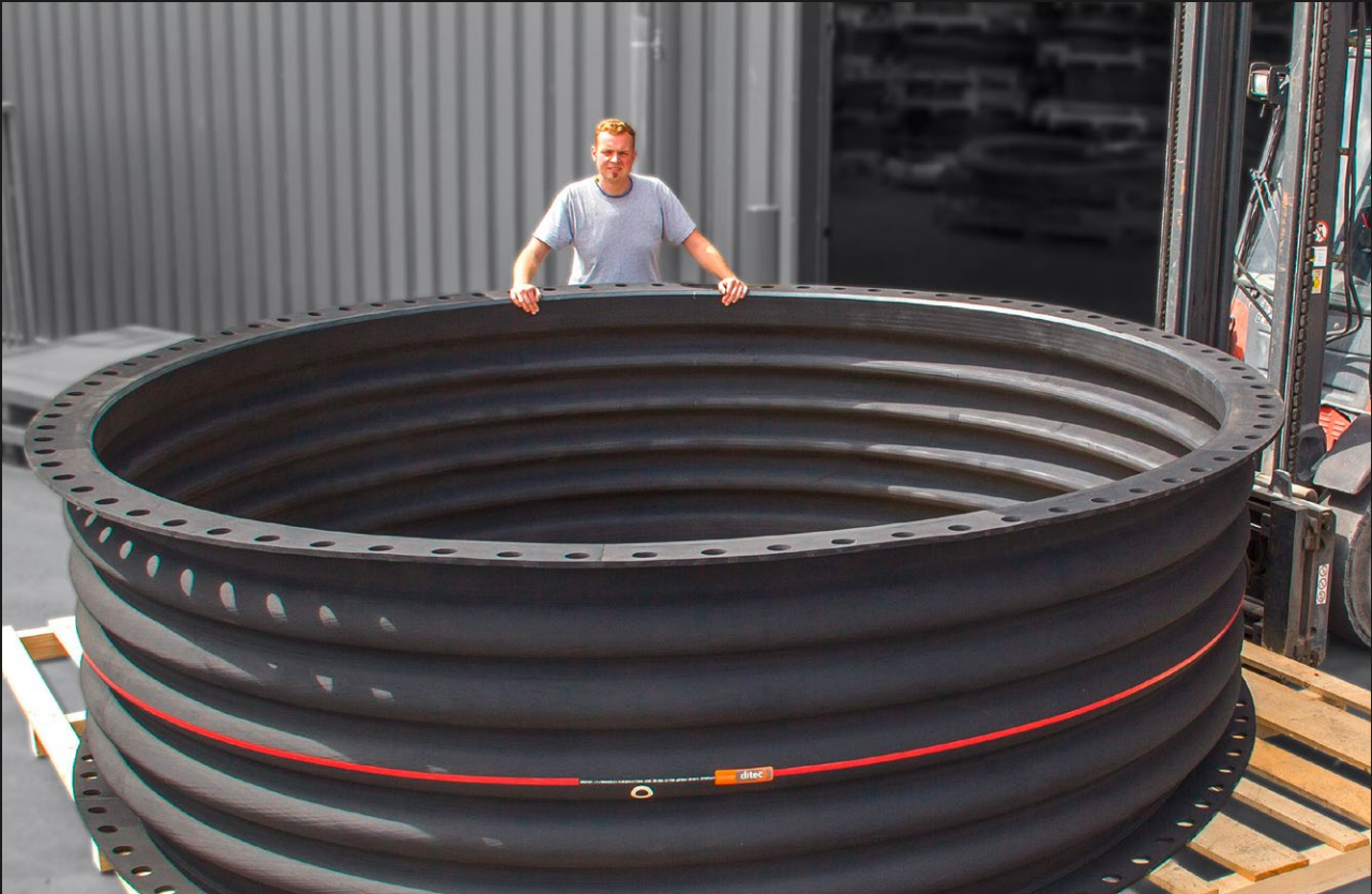
Rubber expansion joint with five arches of size \varnothing 3,600 mm for a submerged cooling water intake line
