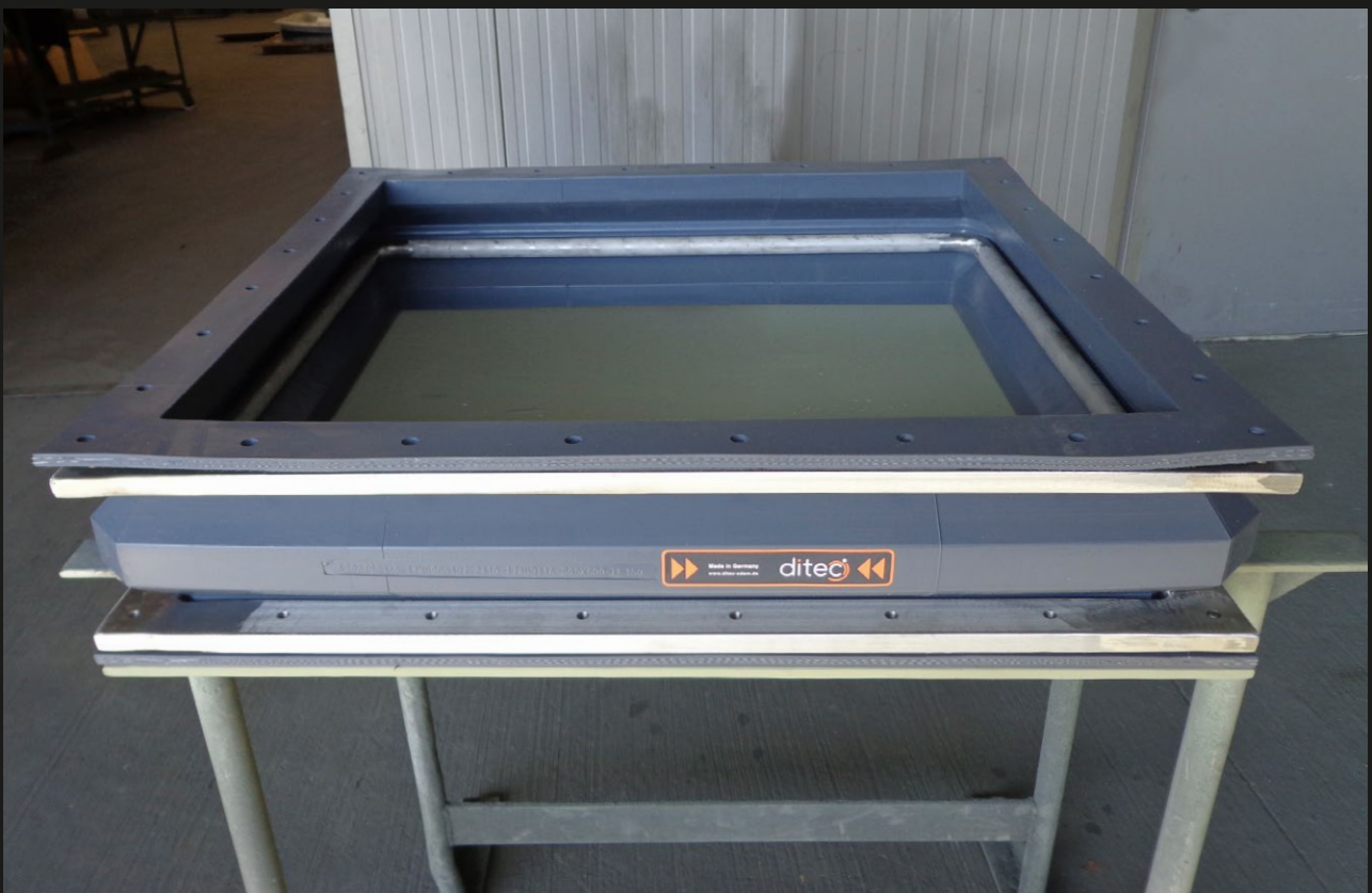
Radiation resistant Silicone single arch rubber bellow with internal vacuum ring prepared for hydraulic testing installation on a high-pressure fan inside of a nuclear power plant
