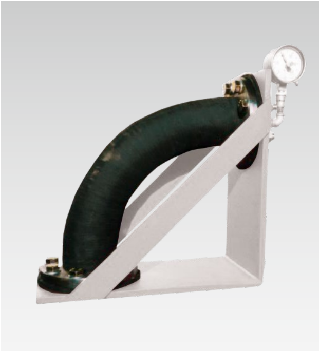
Rubber bend in pressure test \varnothing 100 mm, 40 bar
